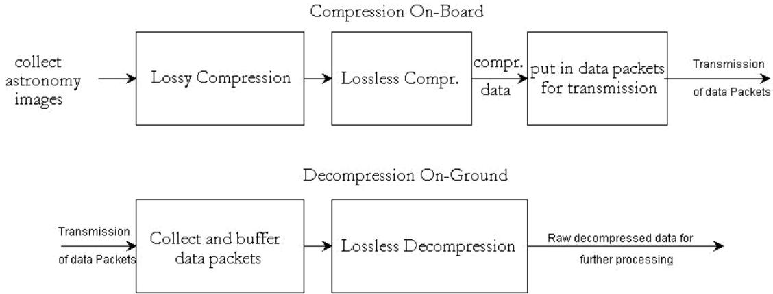
Figure 3: Block diagram of the basic concept
