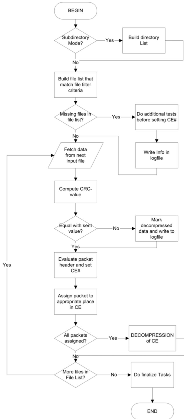
Figure 6: Flowchart of data buffering
