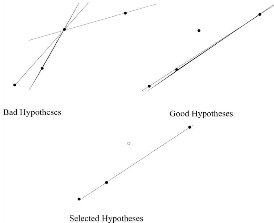
*Figure 3. Illustration of RANSAC*
