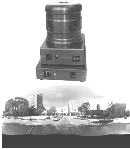
Figure 5: “Ladybug 2” panorama camera from PointGrey (top), and reconstructed panorama (bottom)
