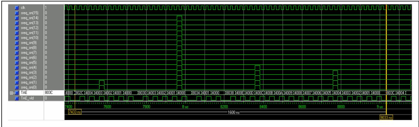
Figure 4. Simulation result for the parameter values:  $f_{clk} = 40$  MHz,  $N_i = \{2, 15, 5, 4, \dots\}$ ,  $T_{TS} = 400$  ns
