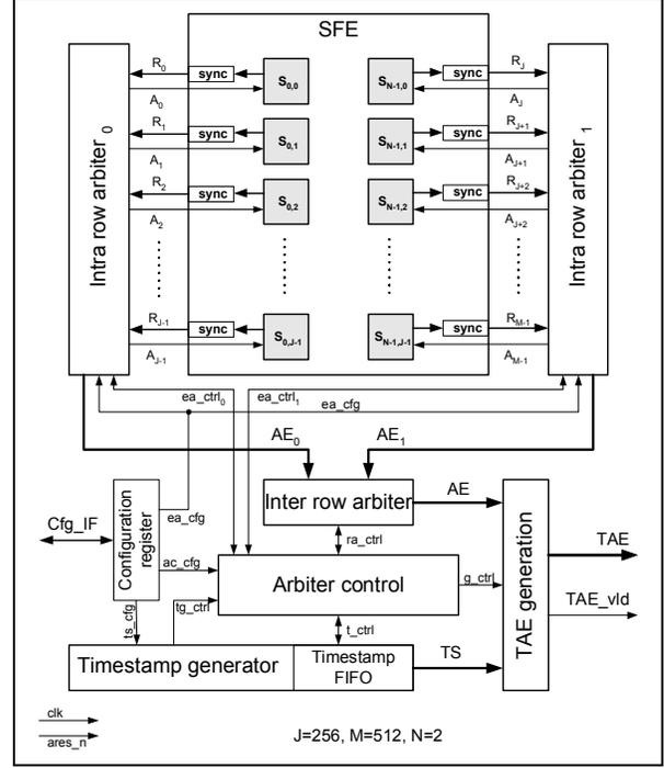
Figure 1. Top level architecture of the arbiter
