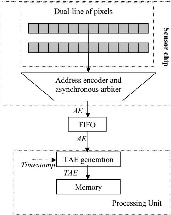
Fig. 1. Address-Event communication periphery using the asynchronous arbiter
