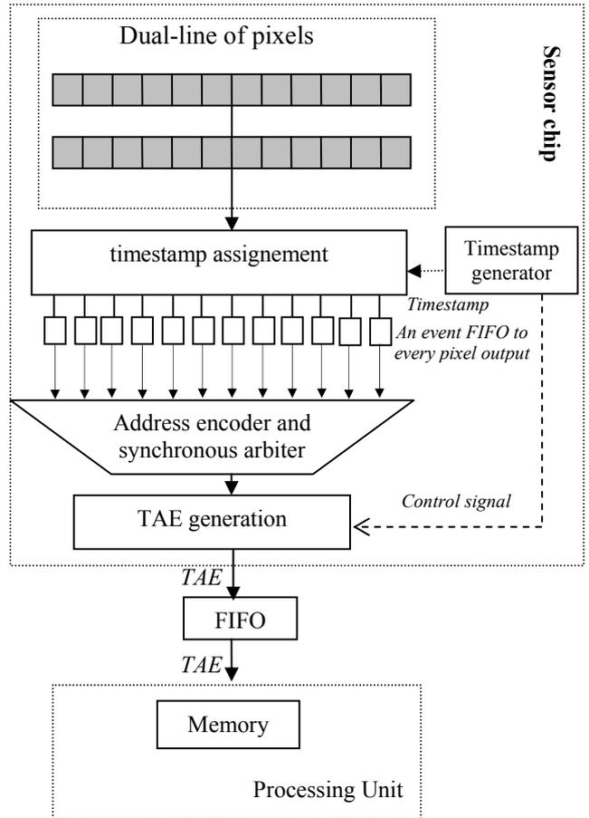
Fig. 2. Address-Event communication using the synchronous arbiter
