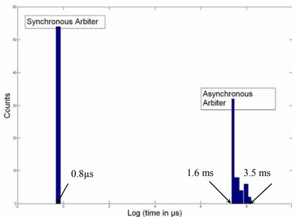
Fig. 4. Histogram of the arbitration duration with the synchronous (left) and asynchronous for several measurements
