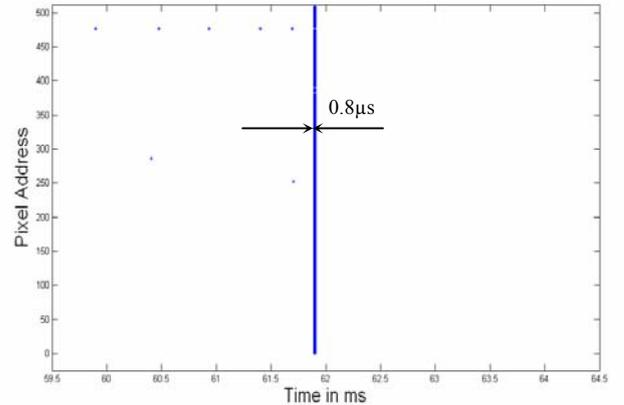
Fig. 3. Dual-line sensor data for the laser light flash using a.) the asynchronous arbiter and b.) the synchronous arbiter
