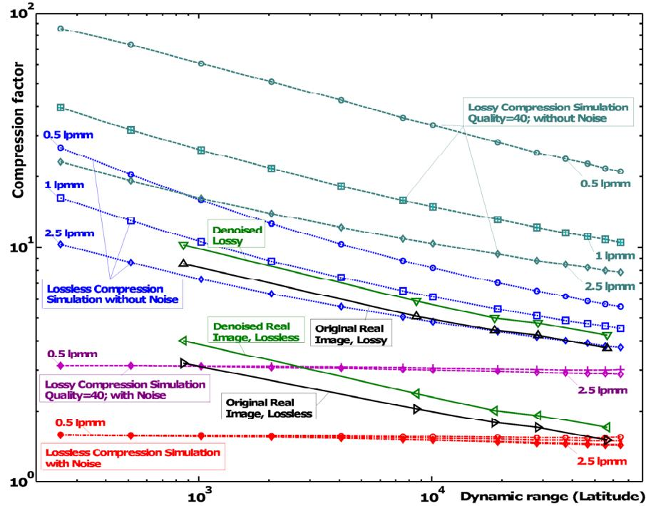
**Figure 1.** The dependency of the compression factor on the dynamic range for smooth noisy images. There are four groups, each showing the three lines-per-millimeter frequencies 0.5, 1 and 2.5 lpmm, for lossless, lossy, lossless with noise and lossy with noise images (see also Table 1).
