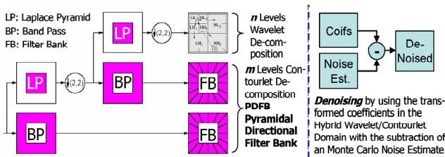
**Figure 2.** The concluded hybrid approach will use the Contourlet transform for the first decomposition levels and the biorthogonal wavelet transform for the lower resolution levels. The ROI and the denoising approach will be extended to the hybrid scheme.
