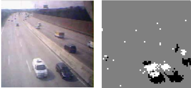
Figure 3: Video frame and rendering of AE data
